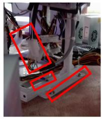
Step5 Remove screws and lift up the mechanism from two sides.
