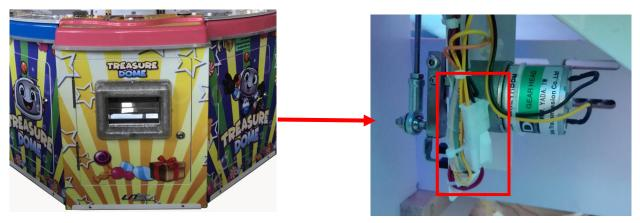
Step2 Locate the latch. Turn latch up to open the door.
