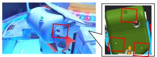
Step 2 Locate the motor and unplug its power cord. Locate the motor gear and utilize 2.5mm Allen Wrench to remove fastening screw. Utilize Phillips screwdriver to remove 3 screws and take the motor out.
