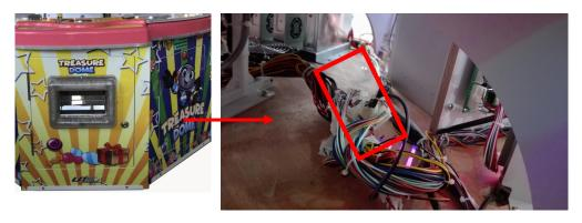
Step4 Unplug the power connector. Utilize Philips screwdriver to remove the GND screw. Utilize 4mm Allen driver to remove the holder screws.
