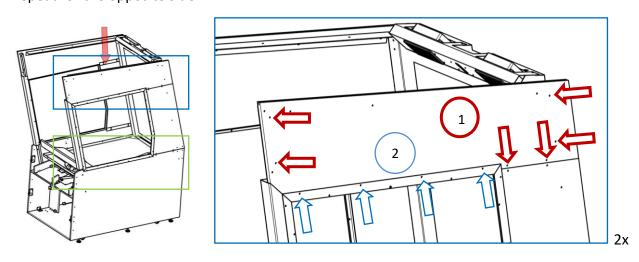
**8)** Install the lower bolts for the window assembly Repeat for the opposite side.
