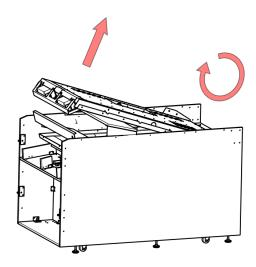
2) Secure the screen into a lifted position using #10-24 x  $1\frac{1}{4}$  philipps bolts. Repeat for the opposite side
