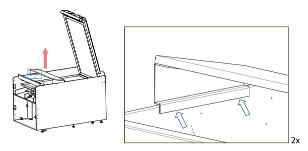
4) Install lateral posts and secure the window assembly with #10-24 x 1% philips bolts Repeat for the opposite side
