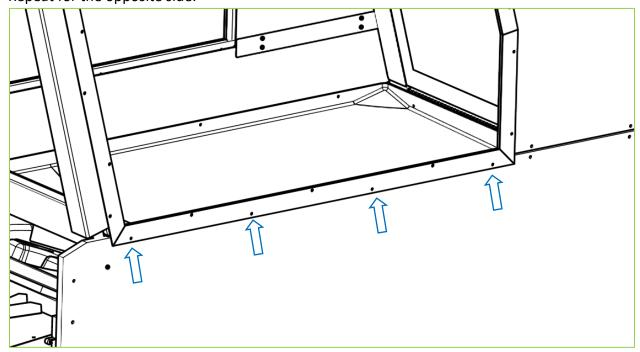
**9)** Assemble the header assembly and top display using Philipps 10-24 x 1% bolts for each side
