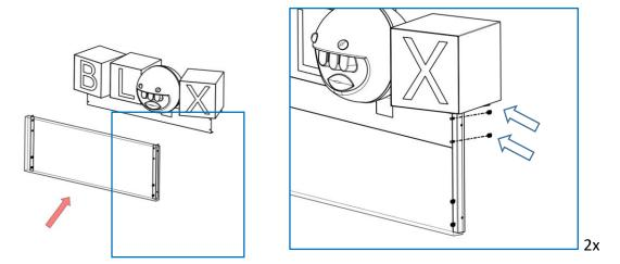
10) Install the header assembly with the upper side panels and Philipps 10-24 x 1% bolts Repeat for the opposite side
