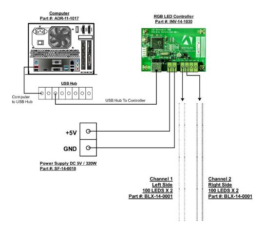
Each side has 2 strips of RGB PCB LED assembly Each strip has 100 LEDs BLX-14-0001
