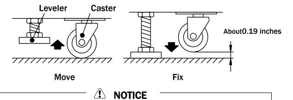
Make sure the machine is level with the ground and all the adjustable legs should stick to the floor closely.
