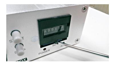
Remove the flathead screwdriver and the SD CARD eject. And then take out the SD CARD.
