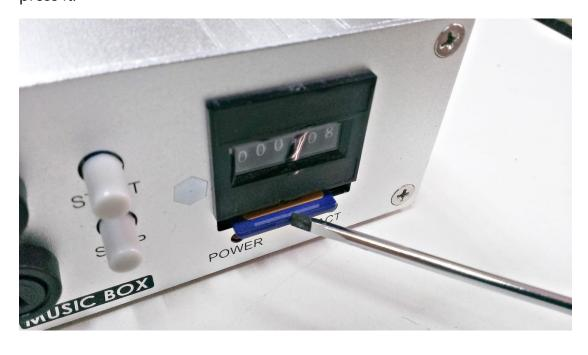
Press to bottom and the SD CARD stuck. The install finished.
