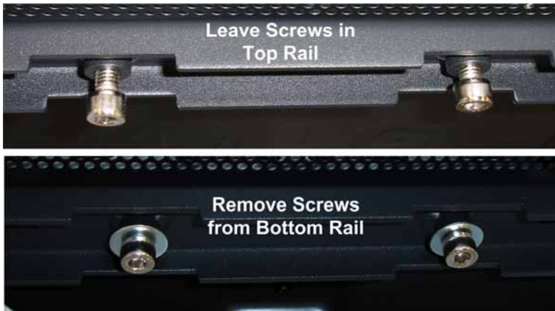
Figure 41. Top and Bottom Rails and Mounting Screws
