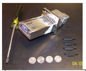
1) Remove the Push Chute from the coin door, and remove the push chute end, proximity plate, anything bolted to the end— for easier access. You will need the Push Chute (of course), enough coins to make it work in its current setting, the inserts for the desired setting, and a Phillips screwdriver.
