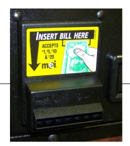
LED OFF – power off LED ON – OK 1 Flash – Bill path jammed 2 Flashes – from system 3 Flashes – Cleaning required 4 Flashes – Cross-Channel Blocked 5 Flashes – Magazine removed Continuous, Slow – Unit Failure – Replace Unit Continuous, Fast – Stacker Full
