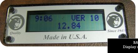
BATTERY QUICK CHECK Display shows time, software version Battery voltage At 12.84v this table's battery is sufficiently charged
