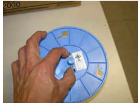
Squeeze the two notches towards center.
