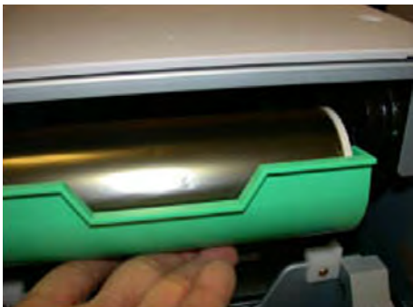
Push the tray up, you will hear a click when the tray is in the correct position.
