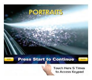
Key Point: To enter configuration mode, simply tap the 6:00 position repeatedly. A keypad will appear in the upper left hand corner of the screen.
