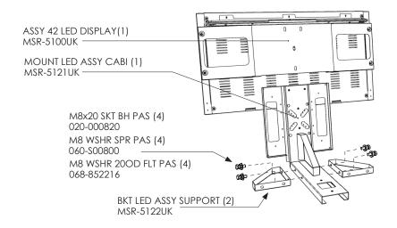
2 Slide the ASSY 42 LED DISPLAY over and onto the MOUNT LED ASSY CABI and secure using (4) M8x20 SKT CAP PAS screws and associated washers.
