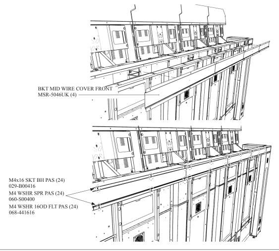
Offer the (2) BKT OUTER WIRE COVER FRONT (MSR-5049UK) individually up to the BKT WIRE COVER REAR on each of the TOWERS. Secure using (6) M4x16 SKT BH PAS and additional washers. where shown.
