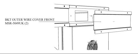
Repeat the above process when attaching the BKT OUTER WIRE COVER FRONT (MSR-5049UK) to the RH TOWER.
