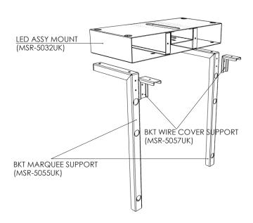
Apply the LED ASSY MOUNT and both BKT WIRE COVER SUPPORTS to the BKT MARQUEE SUPPORT using the fixings shown.
