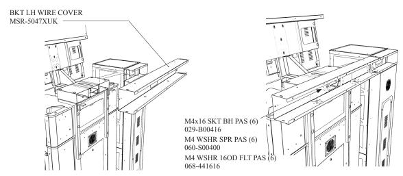
Attach BKT MID WIRE COVER REAR (MSR-5054XUK) to Cabinet 2. (Cabinet 2 BKT MID WIRE COVER REAR has the PI CPU attached to it). using the fixings as shown.
