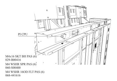
Attach BKT MID WIRE COVER REAR (MSR-5054XUK) to Cabinet 3 and Cabinet 4 in the same way as the BKTS attached in Steps 2 and 3, until all BKT WIRE COVERS have been fitted. Finally apply the BKT RH WIRE COVER REAR to the RH TOWER as instructed in STEP 1.
