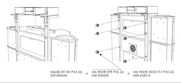
Finally secure the upper section of the LED SUPPORT BKT by fitting (2) M6x40 SKT BH PAS Bolts in locations shown. Proceed to carry out operations 1 to 5 on the remaining 3 cabinets..
