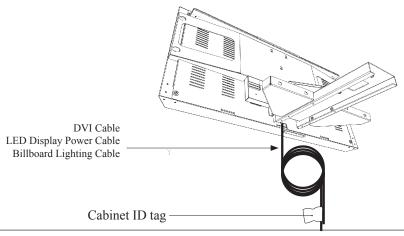
Using a minimum of 4 people and or lifting equipment. Offer the ASSY 42 LED DISPLAY assigned to cabinet 1 up to cabinet 1 and slide it carefully into the LED ASSY MOUNT. Take care not to damage any harnessing when applying the ASSY 42 LED DISPLAY to the CABINET.
