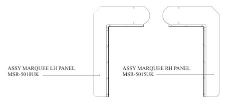
2 Apply the ASSY MARQUEE LH PANEL to the LH Tower. Fix and secure using (8) M4x16 SKT BH PAS machine Screws in locations shown.
