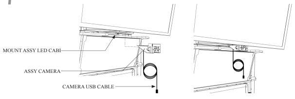
Secure the ASSY CAMERA in place by using (4) M4x16 SKT BH PAS and associated washers..
