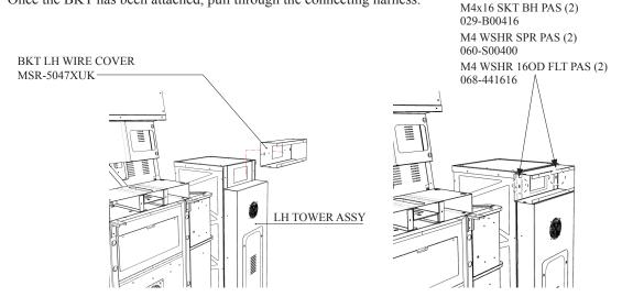
Attach BKT MID WIRE COVER REAR (MSR-5045XUK) to Cabinet 1 and the BKT LH WIRE COVER REAR using the (6) set of fixings as shown.
