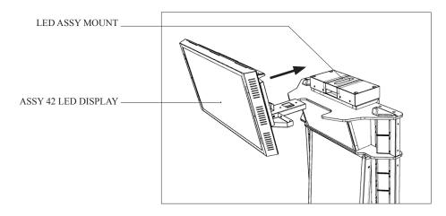
Once the ASSY 42 LED DISPLAY is fully in position, secure to the LED ASSY MOUNT using (6) M8x20 SKT BH PAS and associated washers.
