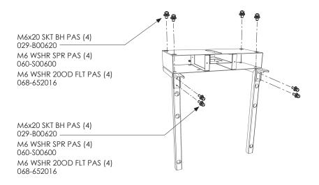
Attach the BKT MARQUEE SUP STRETCHER to the top of each cabinet as shown and secure using fixings M6x20 SKT BH PAS (2), M6 WSHR SPR PAS (2) & M6 WSHR 20OD FLT PAS (2)
