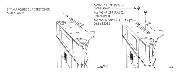
Offer the now assembled LED DISPLAY MOUNT to the top of each cabinet and over the BKT MARQUEE SUPPORT STRETCHER. Once in place secure using the fixings 6 sets of fixings shown.
