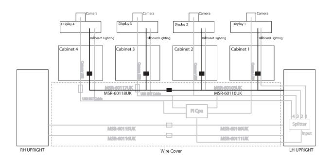
Once all the harness have been applied, secure them into the routers positioned within the BKT WIRE COVERS.
