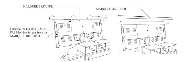
Offer Artwork #1 (MSR-5026UK) to Cabinet 1. Replace the MARQUEE BKT UPPR and re-secure using the (4) M4x12 SKT BH PAS Machine Screws.
