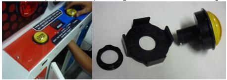
5. Remove the acrylic from the player console by unscrewing both bolts using a 3mm Allen Key.
