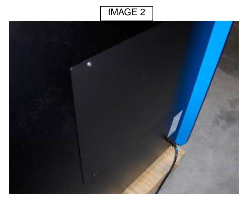
If You Find That The Rear Metal Access Plate Is Bolted Directly To The Game (As Shown In "Image 1" And "Image 2"), Unbolt It And Insert Spacers, Washers, Or Nuts To Separate The Door/Plate From The Game. Be Sure To Evenly Space Each Bolt When Attaching the Rear Access Plate to the Game, So As To Not Bend It. Recommended Spacing Is a ¼" To ½". When Finished The Game Should Look Like "Image 3" And "Image 4".
