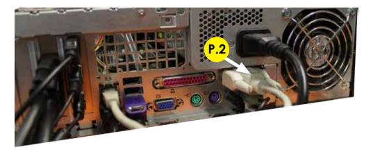
P.2 Control Board. USB to Serial Converter (30cm - Inch 11,8) + Serial Cable to Control Board (100 cm - Inch 39,4)
