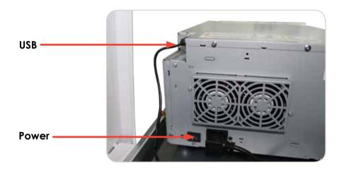
3 · Check the computer connections, USB from printer to PC.
