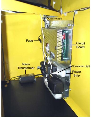
FIGURE 14 CIRCUIT BOARD
