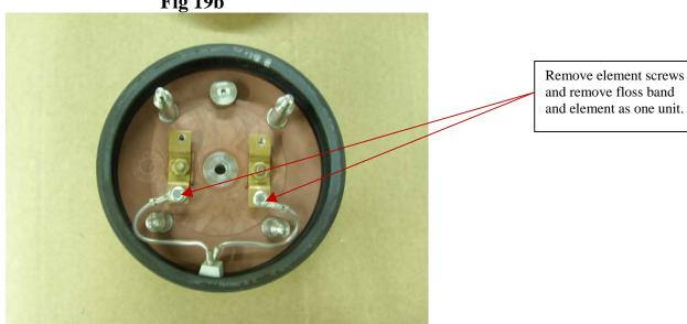
Place the floss band and element in hot water to melt the sugar and release the old element from the floss band. Check the floss band for any external chipping or damage. If any is found then the floss band needs to be replaced. The new heating element will be supplied as shown in Fig 19c. Ensure that the floss band is clean and dry and fit the new element taking care not to damage or stretch it. The leads should be carefully formed around the stainless steel posts as in Fig 19b.
