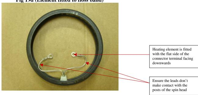
Fit the floss band and element to the base of the spin head. Fit and tighten the element nuts ensuring that the leads and terminals do not make contact with the metal posts. Fit the top cap, washers and nuts. Centralize the floss band assembly in the spin head before tightening the retaining nuts.
