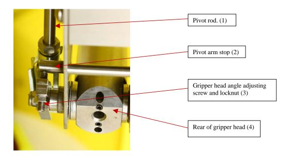
Gripper head. Fig 9b.
