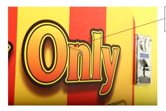
Insert pin or paper clip to depress solenoid plunger. Lift vend door while simultaneously withdrawing the pin.
