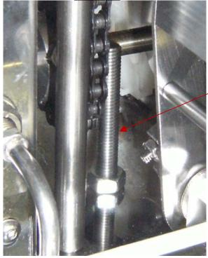
Engage arm adjuster and locknut (3)
