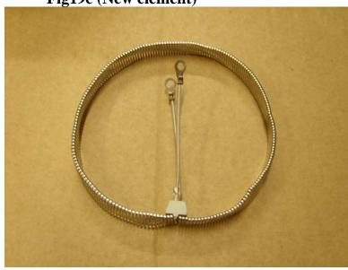
Fig 19d (Element fitted to floss band)
