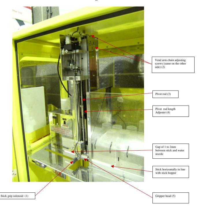
Fig 8. Vend arm mechanism. Home Position (covers removed)
