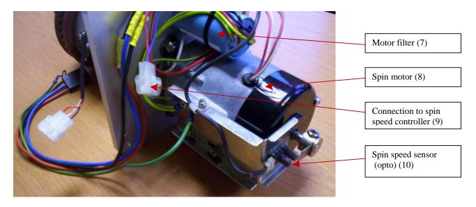
Fig 18a Spin head removed.
