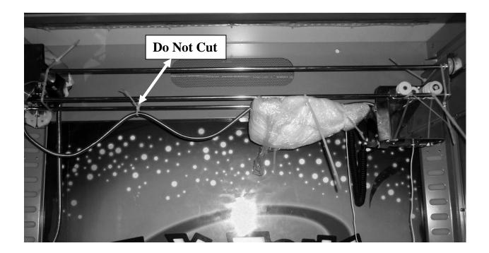
Remove all the cable ties holding the crane and claw secure for transport. Do not cut the cable tie on the central cable ring support
