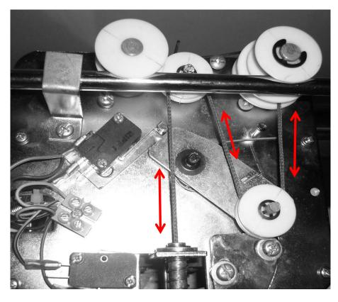
\* **NOTE!** \* Rope length between notches is 1.40 meters (55") maximum.
