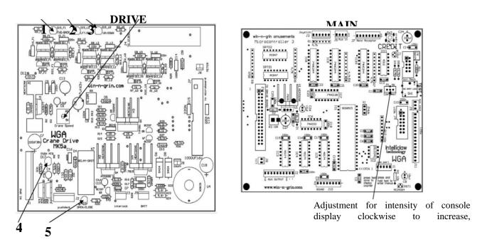
Regulates speed of gantry clockwise faster anticlockwise slower
