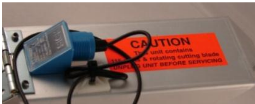
Full Bucket Sensor mounted on Ticket Chute Cover
