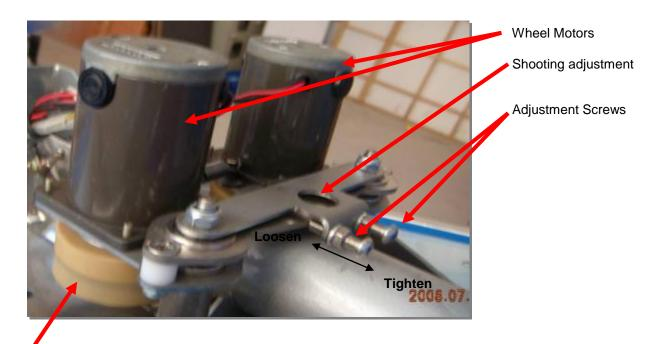
Worn wheels can cause little or no force applied to the ball. Replace if worn.
