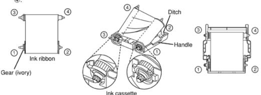
Make sure to set the ink ribbon roller to the ditches firmly. Turn the ivory gear to eliminate any slack.
