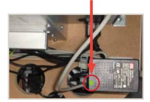
If the power card is properly plugged then the LED is blue.
