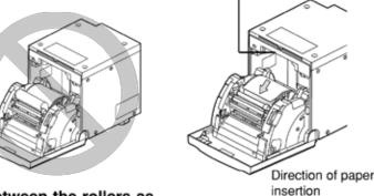
5 Remove the sticker, insert the print paper between the rollers as shown right, and feed the print paper until it reaches the black
