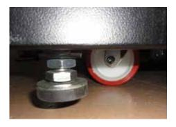
Adjust the height of the four metal legs once the final location for the booth has been established. The metal legs are underneath the cabin next to the wheels.
