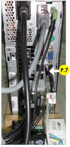
P.7 Dongle USB Security and Software. MEGA OUT
