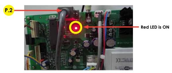
P.2 Serial Cable From Control Board to PC. (56 cm - Inch 22,04)
