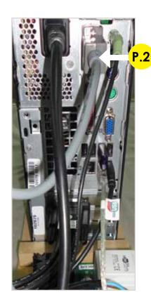
P.2 Serial Cable From Control Board to PC. (56 cm - Inch 22,04)
