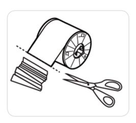
When the manual feed & cut mode has been selected, hold down the FEED & CUT button for 1 second or longer. Repeat the manual feed & cut three times. When the print paper with the postcard printing on its reverse side is installed, repeat this procedure five times.
