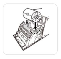
Install the print paper into the unit. Make sure to install the print paper firmly.
