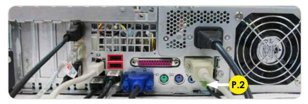
P.2 Control Board. Serial Cable From PC to Control Board M/F. (56 cm - Inch 22,04)
