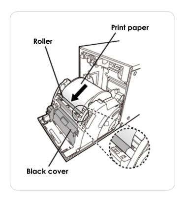
Remove the sticker, insert the print paper between the rollers as shown above, and feed the print paper until it reaches the black cover.
