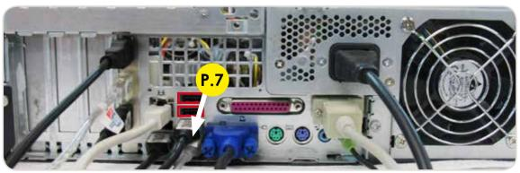
P.7 Dongle. USB Extension AM/AF From Dongle to PC. (180 cm - Inch 70,87)
