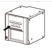
Press the DOOR OPEN button to open the door. Take the ink cassette in the printer out.
