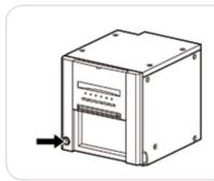
Press the POWER button to turn on the power.
