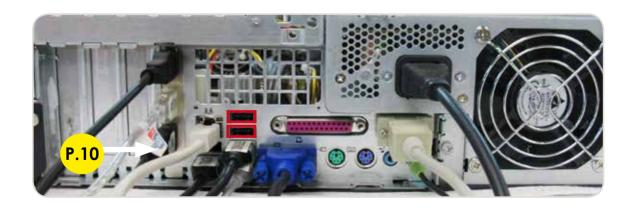
P.10 Camera. USB Extension AM/AF From Camera to PC. (180 cm - Inch 70,87)
