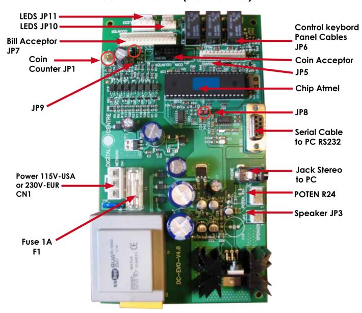
RS232. Serial Cable. From Control Board to PC.
