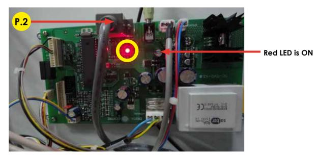
P.2 Control Board. Serial Cable From PC to Control Board M/F. (56 cm - Inch 22,04)
