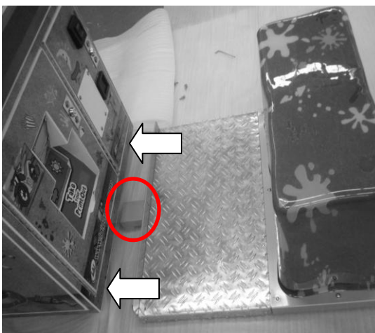
Position the seat aligned with the cabinet with the middle bar in center of cabinet
