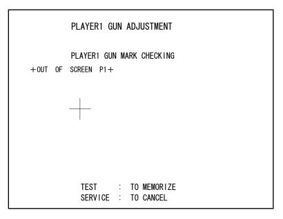
Point the Control Unit (Gun) at the screen and a gun mark will be displayed. Check to make sure that the gun can aim right up to the edges of the frame.
