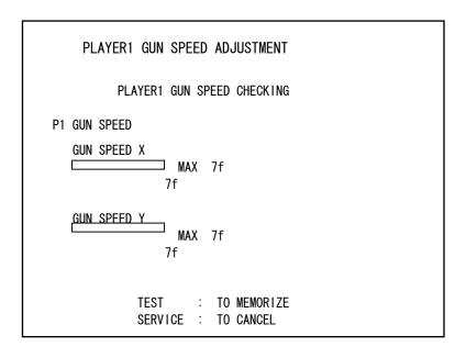
The set MAX speed values will be displayed. Move the gun again and check that these are no problems with these speed settings. If everything seems in order, press the TEST Button.
