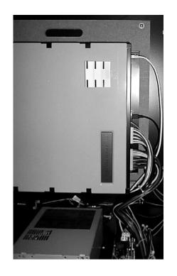
Secure DLP and GUN Cabinets together using 2x M8x30 Hex Bolt and 2x M8x65 Hex Bolt
