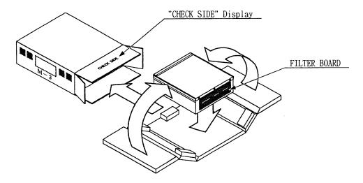
Wrap the ASSY GAME BOARD with the packaging material and put it in the original transit box as shown. Putting it upside down or packing otherwise in the manner not shown can damage the GAME BOARD and parts.
