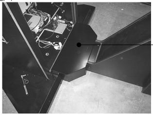
Remove the JOINT COVER (HDF-1031UK) from over the joint of the 2 cabinets (2x M5x16 PAN PAS BLK and 2x M6x50 HEX BOLT BLK.)
