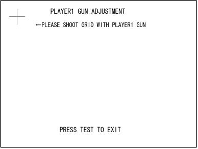
Follow the on-screen instructions to adjust the gun sight settings. Aim at the mark in the upper left corner and fire. The mark in the upper left will disappear, and the same mark will be displayed in the lower right corner.
