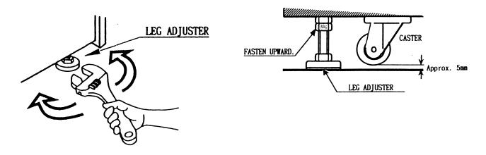
After securing the leg adjuster bolts, fully tighten all bolts temporarily attached in steps 1 above. Ensure adequate ventilation and operating space is maintained as detailed below.
