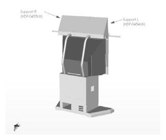
Place the BILLBOARD PLATE (HDF-0453UK) on the back of the SUPPORTS L&R and secure along the bottom edge using 4x M6x12 MCSR PAN W/FS PAS.
