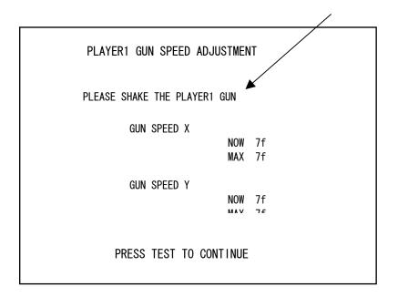
Follow the onscreen instructions to perform the gun speed settings. Shake the gun on the X axis and the Y axis and set the MAX value for each.
