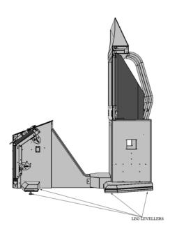
Ensure that the LEG LEVELLERS are raised above the position of the CASTORS before attempting to move.
