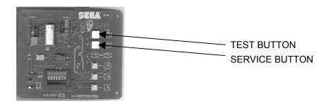
Opening the Coin Chute door will reveal the VTS Assembly shown above. The function of each switch is as follows. The controls on the left affect the 1P cockpit, those on the right the 2P.
