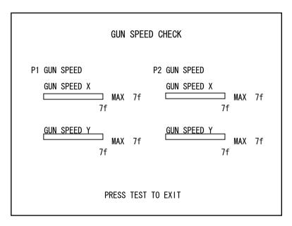
Moving the gun for each player will alter the values displayed on the X axis and Y axis speed bars. Use this screen to check that the current maximum speed setting matches the speed values by moving the guns around.
