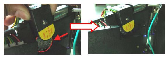
Step15: Check the Coin Acceptor Setting. (Select "NO" on top switch, "SLOW" on bottom switch)
