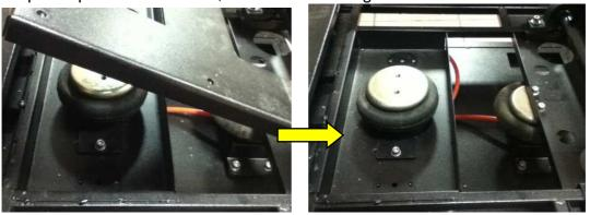
Step5: Remove 2 fixation screws.
