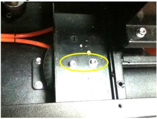
Step3: Remove 4 fixation screws.
