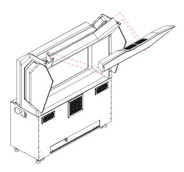
Carefully move the TV cabinet (monitor base) close to the Cockpit (seat base).
