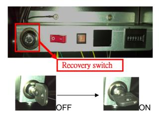
**Step1:** When the screen shows "insert coin", Use the key specified for recovery switch and turn it right.
