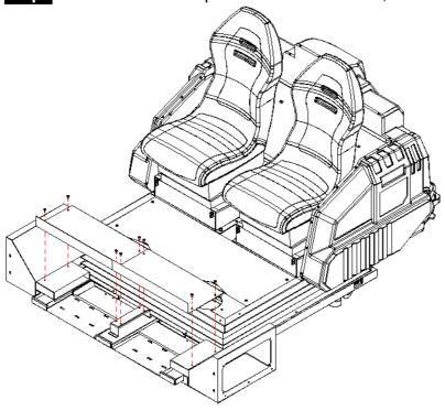
Step9: Attach the cover plates to the connector boxes, and use the screws to fix it.
