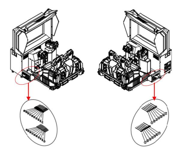
Step4: Collect the connectors ①~⑦ from TV cabinet to the connector box on Cockpit right hand side by the same pin-number and the same name tag.
