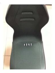
Step3: Remove 2 airbag screws.
