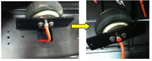
Step7: After changing, lock 2 airbag screws, tube, and 2 fixation screws.
