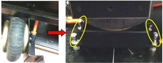
Step9: Install 2 airbag screws. <Finish>
