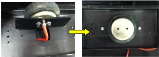
Step8: Cover the seat base, tighten 2 airbag screws.
