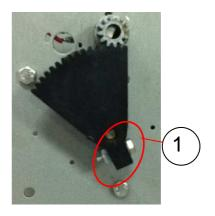
Step8: Use meter to measure resistance value between pin2 and pin3 of the potentiometer. <Finish>
