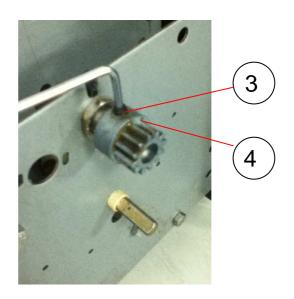
Step6: Install gear2, and make sure gear4 close to second tooth of the gear2.
