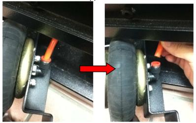
Step5: Remove 2 airbag screws and quick coupler.
