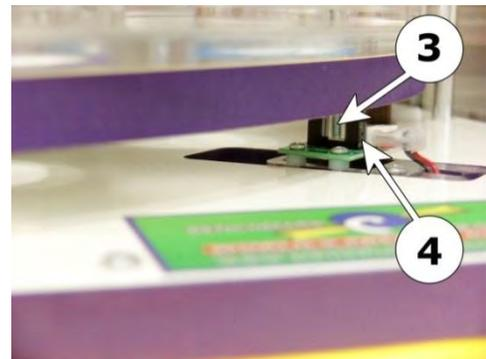
Since the computer knows where the pin in the wheel is relative to each hole position and it knows how many motor steps from home to each hole, we know exactly which hole the ball fell through allowing a payout accurately corresponding to the hole position.
