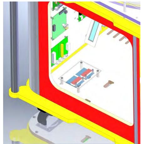
Attach the bracket to the board. Then connect the Emulator bracket harness to the game using the 8 pin microfit connector located above the power distribution board.
